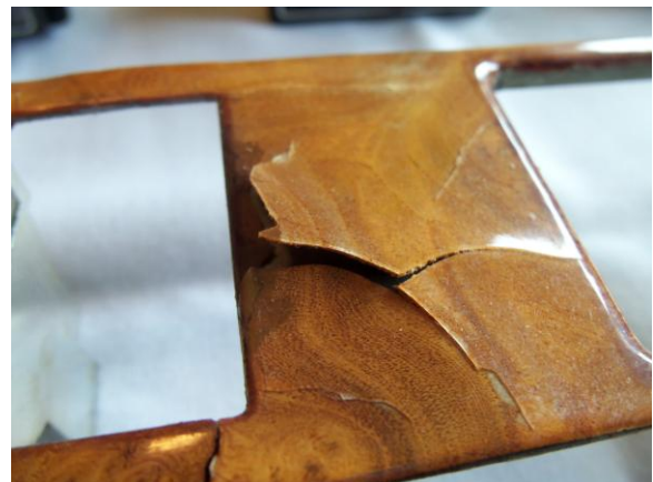
Almost none of the veneer is still adhered to the metal back in this part between the left switches and the clock to the right.
