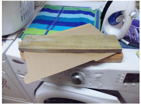
Ready for overnight clamping overnight and flattening of the wood veneer.
