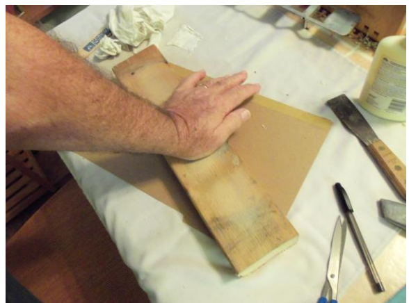
Applying initial pressure to set the veneer into the glue prior to clamping.
