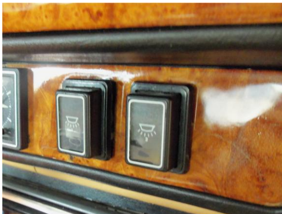
This is a close up of the installed wood veneer, you can see some of the crack lines behind the clear lacquer, but it is all flat, smooth, and glossy.
