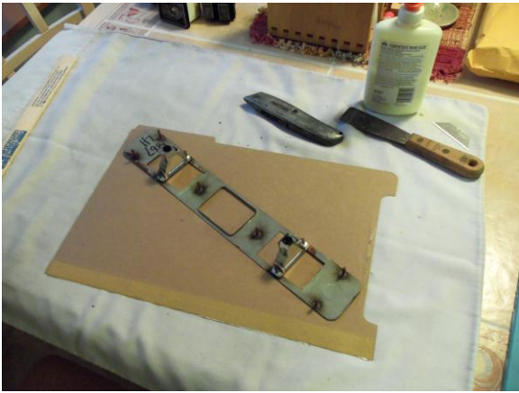
Tracing the metal backing to make the cardboard backing for the wood veneer.
