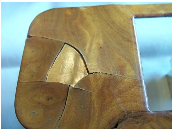
The center piece of veneer fell out when the switches and clock were removed.
