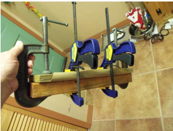
Clamps applied to flatten the wood veneer while clamping for gluing to the cardboard backing.
