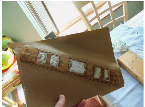
Wood veneer after being clamped overnight to glue the wood veneer to the cardboard backing and flatten the wood veneer.
