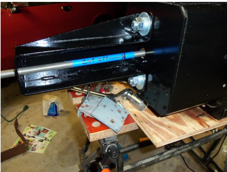
Showing the length the threaded rod will be cut to match the retracted 1-13/16-inch length, measured with the original threaded shaft of the hydraulic cylinder.
