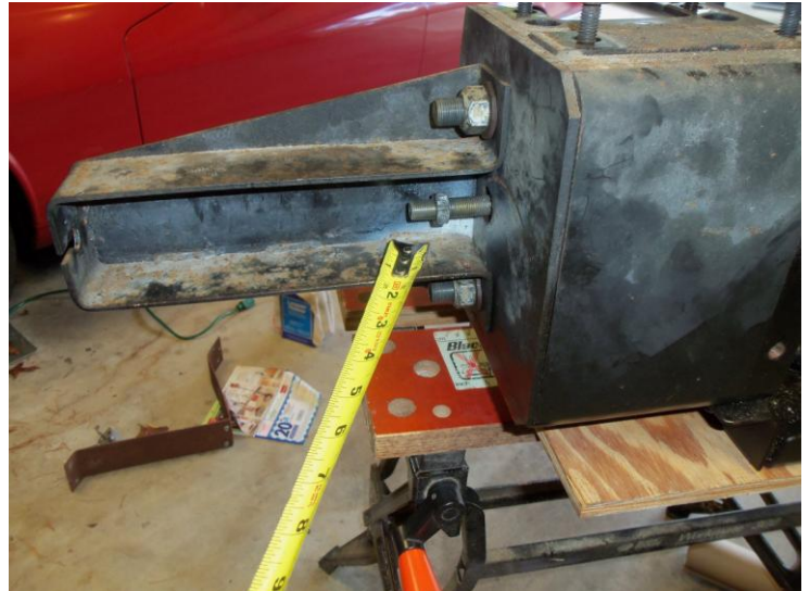
The threaded shaft, which projects out of the hydraulic cylinder and onto which the coupling nut was threaded.
