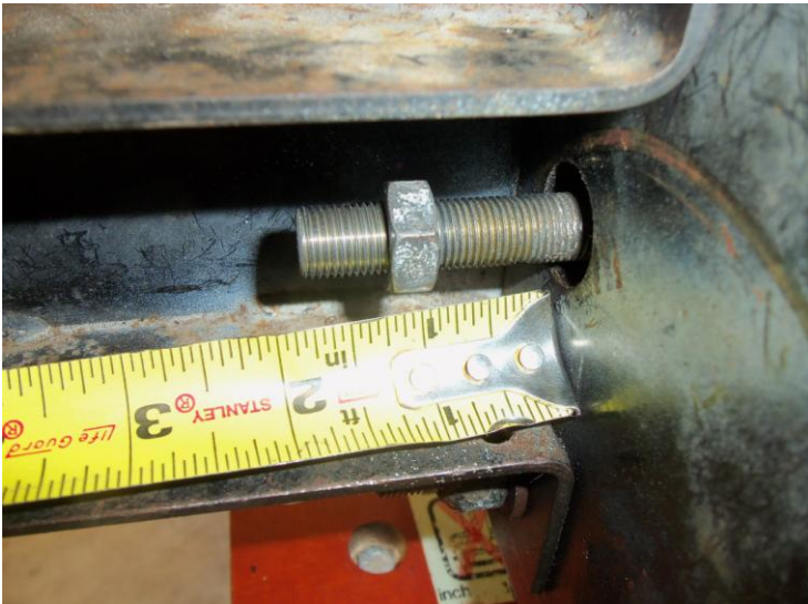
Measure the distance from the end of the threaded shaft to the front plate, as the bolt of the new operator will need to be the same length. The end of the threaded shaft of my hydraulic cylinder measured 1-13/16 inches from the front plate when fully retracted.
