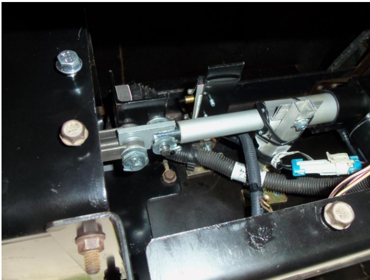
The installed park brake unit with the actuator extended (brake off).
