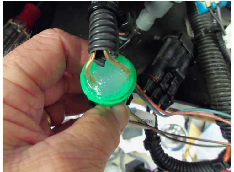
After soldering the wires to the contacts and making sure the connections were good, I filled the switch body with dielectric sealant.
