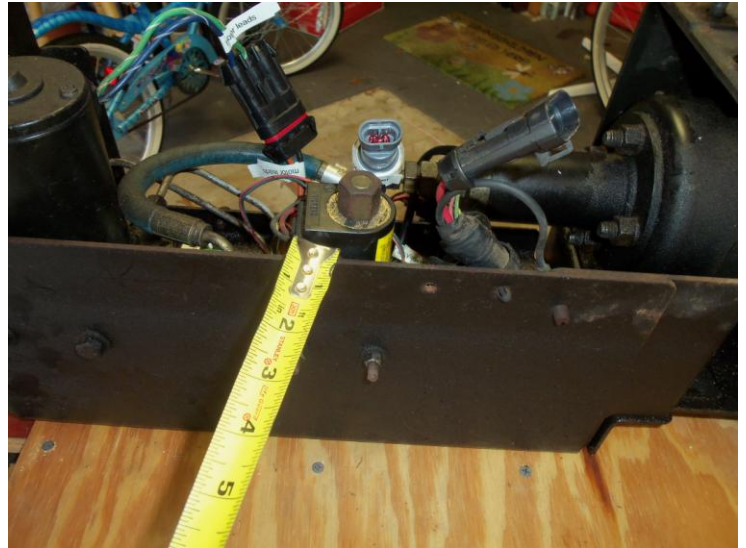
The dump valve, which will be removed.
