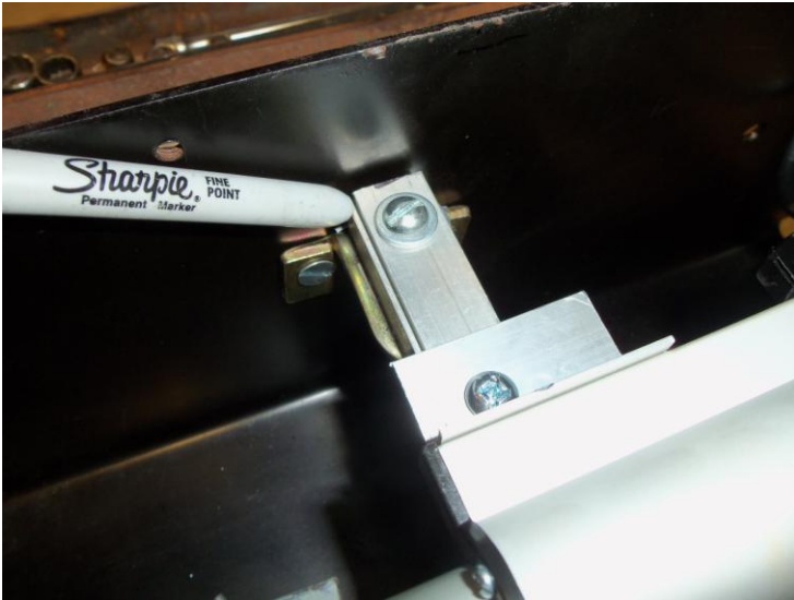
The actuator support bracket is mounted to the MB3 bracket attached to the side of the unit's box.
